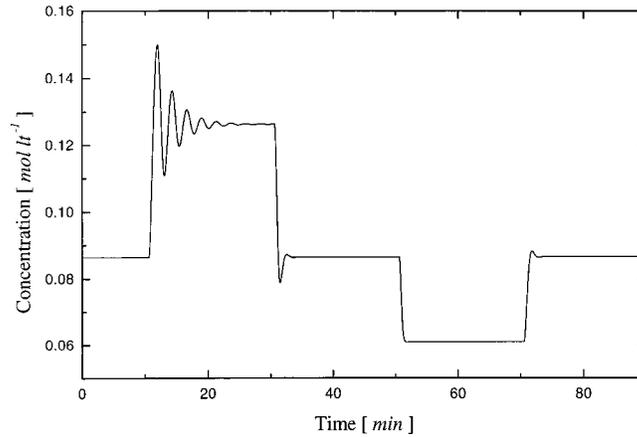
Fig. 9. Open-loop responses of the CSTR concentration to step changes in the coolant flow rate  $q_C(t)$ .
