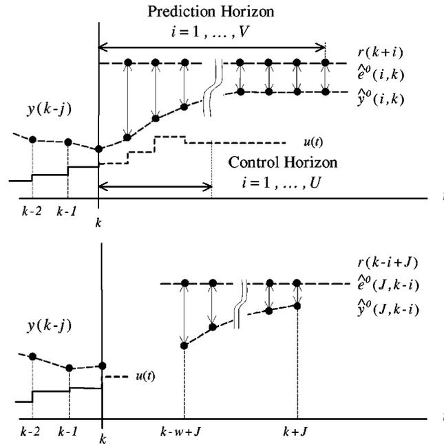
Fig. 5. General MPC and predictive feedback setups.
