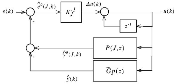
Fig. 1. Structure of the single-prediction controller.
