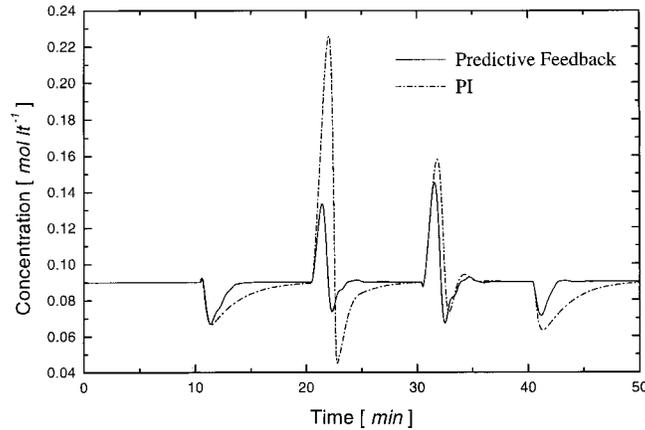
Fig. 12. Closed-loop responses of the CSTR concentration to a sequence of load changes using the predictive controllers.
