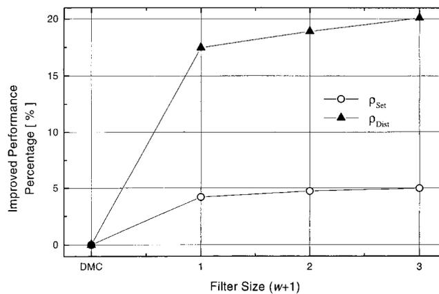
Fig. 8. Performance comparison between DMC and predictive feedback using the ISE index.
