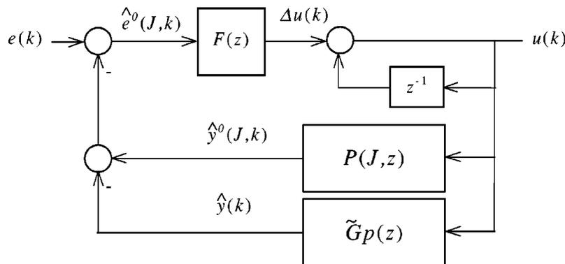
Fig. 6. Structure of the predictive feedback controller.
