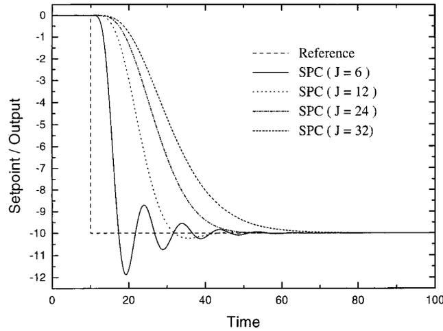
Fig. 2. Closed-loop responses of the linear system to a step change in the setpoint, showing the effect of the prediction time  $J$ .
