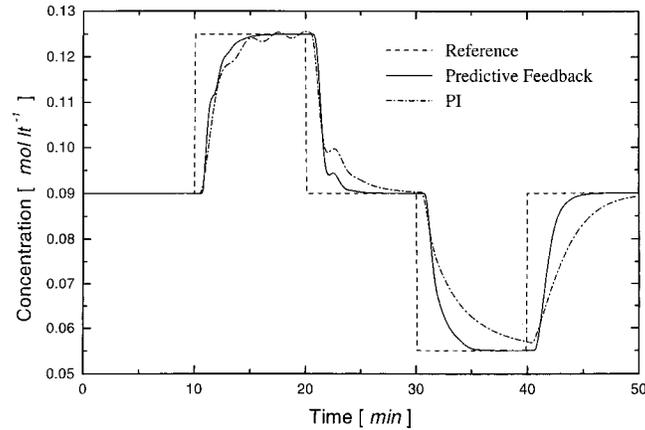
Fig. 10. Closed-loop responses of the CSTR concentration to a sequence of step changes in the setpoint using the predictive controller with one-side constraint in the manipulation and a PI controller adjusted with ITAE.
