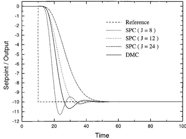
Fig. 4. Closed-loop responses of the linear system to a step change in the setpoint, comparing the response of the DMC and single-prediction controllers.
