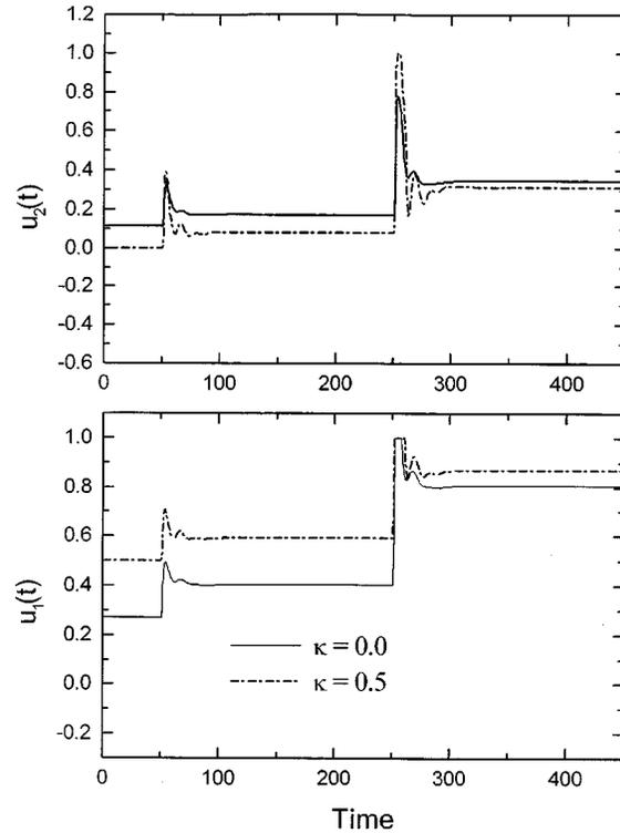
Fig. 12. Primary and auxiliary variables corresponding to set-point and disturbance changes of Fig. 11.
