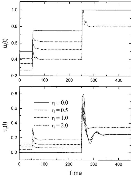
Fig. 10. Primary and auxiliary variables corresponding to set-point and disturbance changes of Fig. 9.
