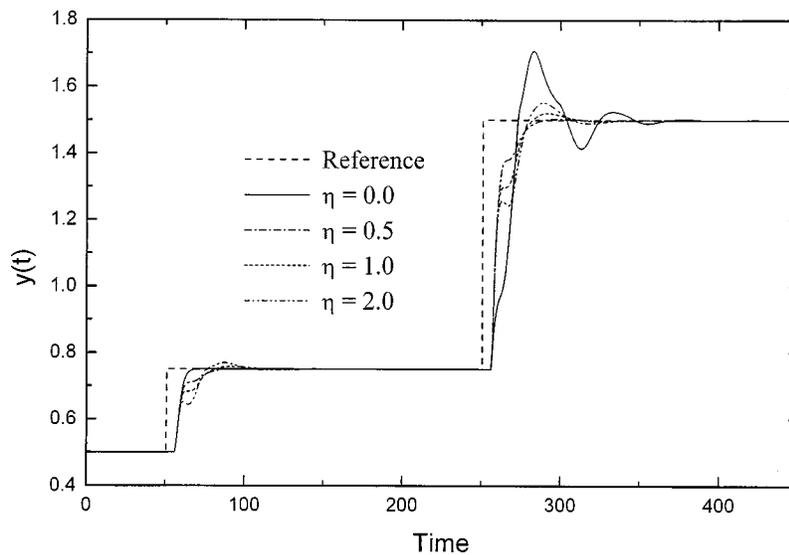
Fig. 9. Set-point responses obtained for different values of  $\eta$ .
