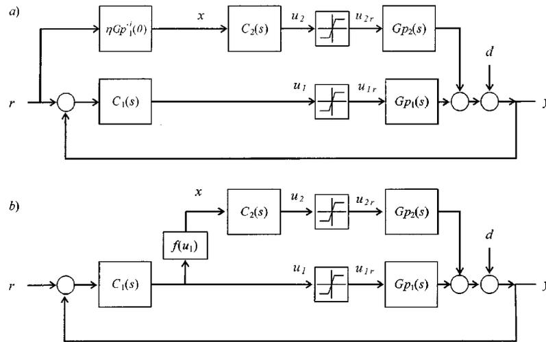
Fig. 2. Block diagram of (a) preventive protection, and (b) reactive protection.
