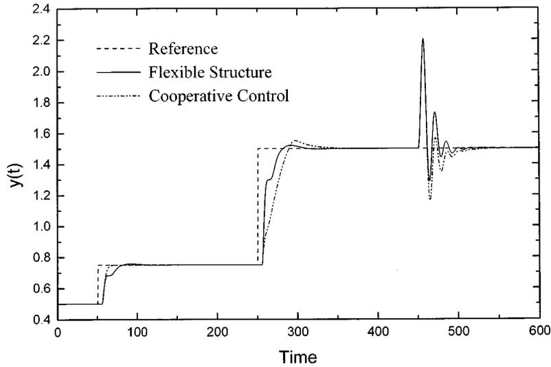
Fig. 7. Set-point responses obtained using flexible structure and cooperative control.
