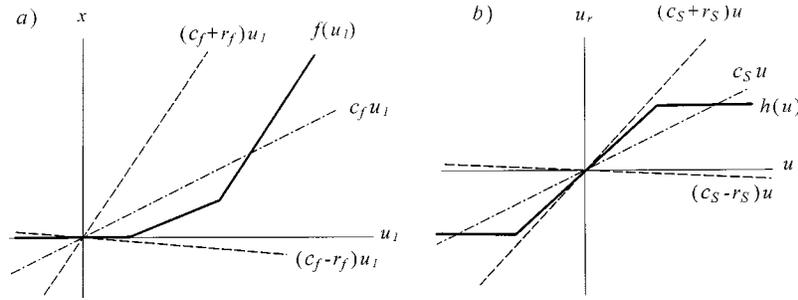
Fig. 5. Nonlinearities and its approximations for stability analysis: (a) decision function, and (b) saturation.
