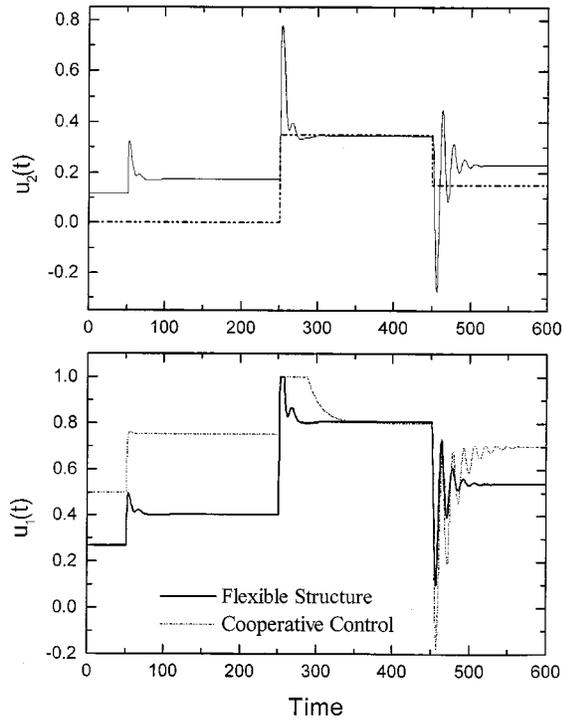
Fig. 8. Primary and auxiliary variables corresponding to set-point and disturbance changes of Fig. 7.
