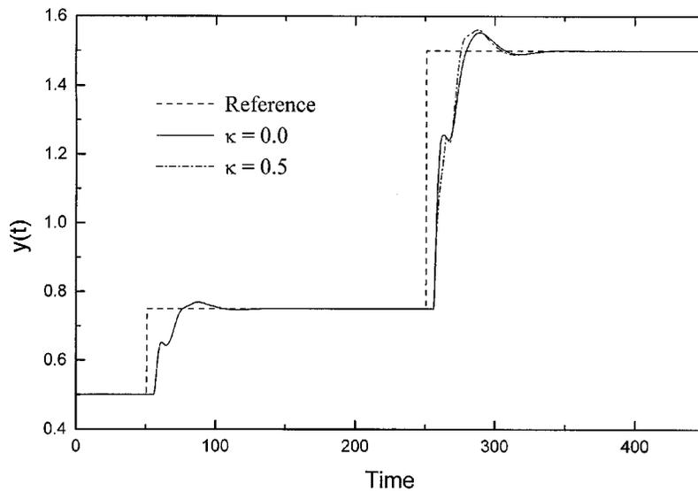
Fig. 11. Set-point responses obtained for different values of  $\eta$ .
