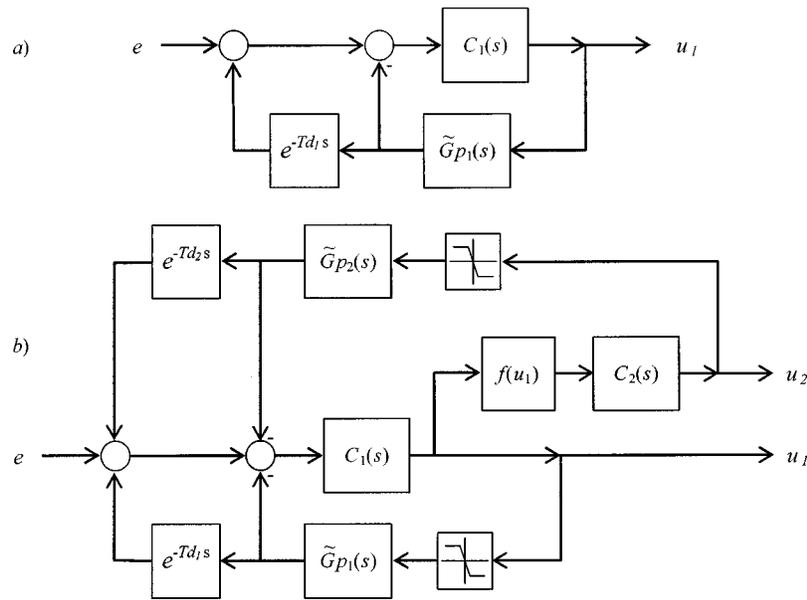
Fig. 4. Block diagram of Smith predictor (a) for normal system, and (b) for cooperative control.
