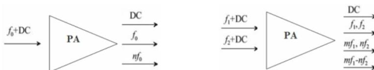
Figure 2.12. Power Amplifier with one-tone (left) or two-tone (right) input signal: harmonics generation.
